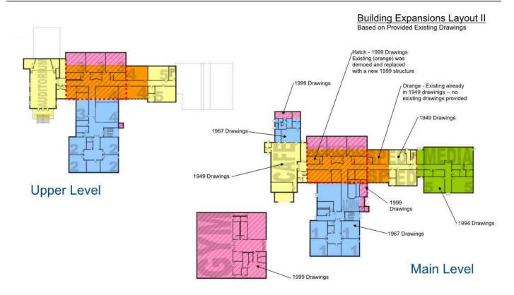
Plan Diagram of Existing Buildings and Expansion Joints
