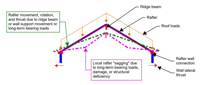
Sketch 1: Roof System Load Path and Lateral Thrust Diagram
